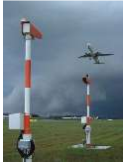
Transmissometer RVR 40 remaining in US
